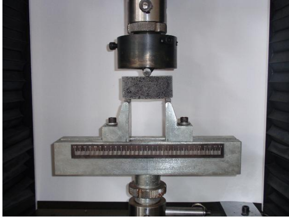
Fig. 8. Fracture test set-up for conducting mixed mode I/III experiments.
