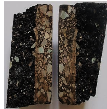
Mixed mode I/III ( \alpha = 30^\circ )
