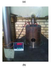
**Fig. 1.** (a) A general view of the ECAE die, (b) Avery universal testing machine.
