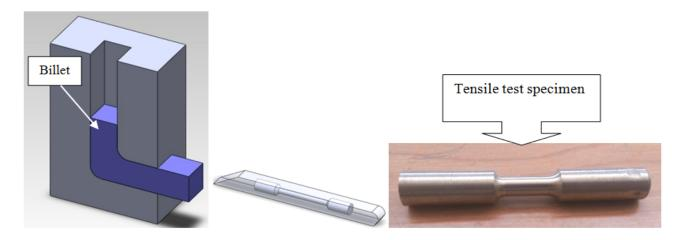
Fig. 2. Fabrication of tensile test specimens from the extruded materials.
