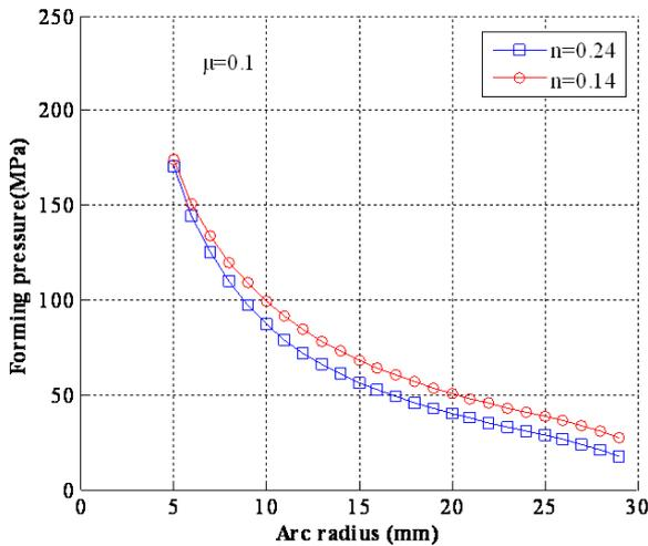
**Fig. 7.** Effect of the strain-hardening exponent on the forming pressure for  $r_0 = 30\text{mm}$ ,  $t_0 = 2\text{mm}$ ,  $R = 1$ .
