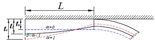
**Fig. 2.** Thickness variation along contact length for frictionless ( $\alpha = 0$ ), sticking ( $\alpha = 1$ ) and intermediate friction cases ( $0 < \alpha < 1$ ).
