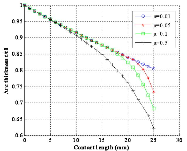
Fig. 5. Change in arc thickness for various friction coefficients for  $r_0 = 30\text{mm}$ ,  $t_0 = 2\text{mm}$ ,  $R = 1$ .
