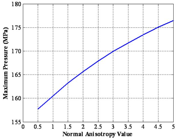
**Fig. 8.** Effect of the anisotropic value on the forming pressure for  $r_0 = 30\text{mm}$ ,  $t_0 = 2\text{mm}$ ,  $\mu = 0.05$ .
