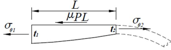
**Fig. 3.** Free body diagram of the stresses acting on tube contact length  $L$ .
