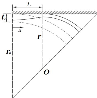
**Fig. 1.** One-eighth of the initial (dashed line) and deformed tube (continuous line).
