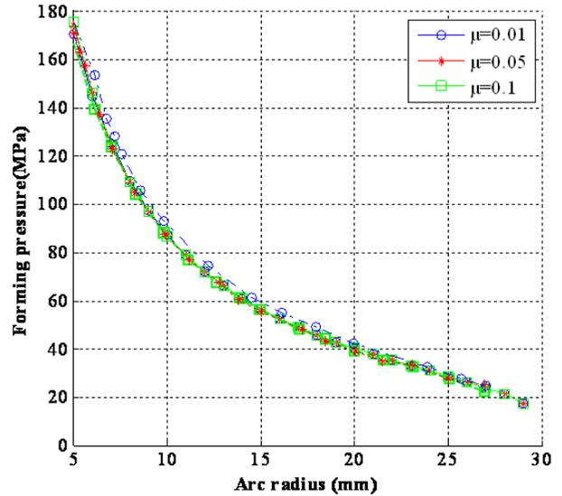
Fig. 4. Variation of forming pressure with arc radius for various frictions and  $r_0 = 20\text{mm}$ ,  $t_0 = 2\text{mm}$ ,  $R = 1$ . (Comparison between predicted values, continues line, and those of Ref. [8], dashed line)
