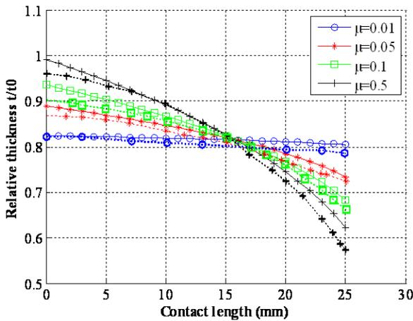
**Fig. 6.** Comparison of predicted thickness variations (continues lines) and values of Ref. [8] (dashed lines), for  $r_0 = 30\text{mm}$ ,  $t_0 = 2\text{mm}$ ,  $R = 1$ .
