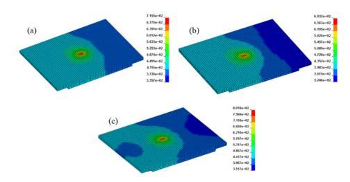
**Fig. 8.** Thermal field in three different modes (according to Table 2) of welding: a) Mode 1, b) Mode 2 and c) Mode 3.
