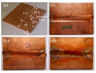
Fig. 1. a) The primary samples, b) Welded piece according to the first conditions on Table 2, c) Welded piece according to the second conditions on Table 2, d) Welded piece according to the third conditions on Table 2.
