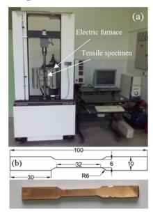
Fig. 5. a) Tensile testing machine and furnace installed on it b) Standard samples of tensile test.
