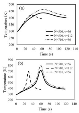
Fig. 9. a) The thermal history in the part of work pieces whose thermal history was experimentally measured and b) The thermal history in the part on which the heat source passes and places in the middle of the intersection line of two pieces (N(rpm), v(mm/min)).
