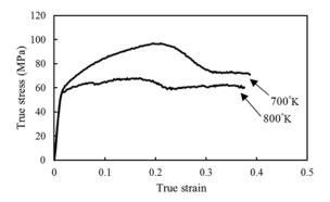
Fig. 6. True stress-strain diagram of the base metal at various temperatures.
