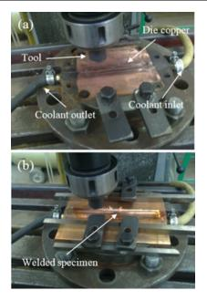
**Fig. 2.** a) A view of the used die and tools, b) Pieces trussed in the die after doing the process.
