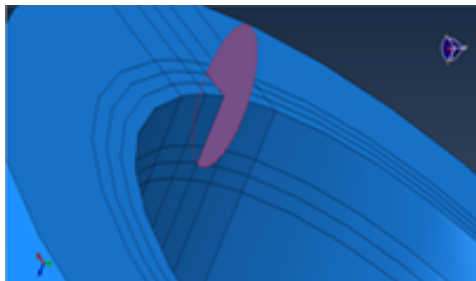
Fig. 10. Internal pressure and boundary conditions on model.
