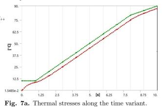
The Fig. 7a represents the temperature distribution of two layers varying with the time obtain using ANSYS which is very much analogous to the temperature distribution obtained in Fig. 6b for various fixed Heat Production in a Simply Supported Multilayer Elliptic Annulus Composite Plate and Its Associated Thermal Stresses: 55–67
