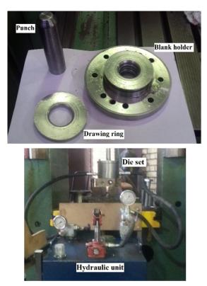
**Fig. 3.** Experimental equipment for hydromechanical deep drawing of a bilayer conical cup.
