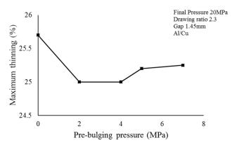
Fig. 15. Effect of pre bulge height on maximum thinning of a bilayer conical cup.
