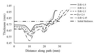
**Fig. 17.** Thickness distribution of Copper for different drawing ratio with constant condition. Final pressure= 20MPa, Pre-bulging pressure= 4MPa.
