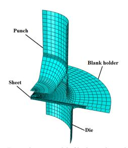
**Fig. 1.** Finite element model of hydromechanical deep drawing of a conical cup.
