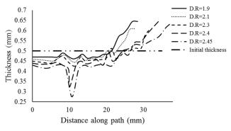
**Fig. 18.** Thickness distribution of Aluminum for different drawing ratio with constant condition. Final pressure= 20MPa, Pre-bulging pressure= 4MPa.
