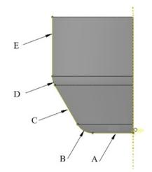
Fig. 10. Different regions of final conical cup.
