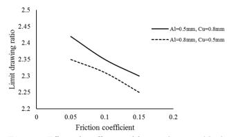
Fig. 13. Effect of coefficient of friction between blank holder and sheet on LDR of a bilayer conical cup (numerical simulation).
