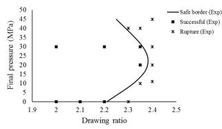
**Fig. 7.** Working zones extracted from experimental tests for a bilayer conical cup.
