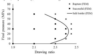
Fig. 6. Working zones extracted from numerical simulations for a bilayer conical cup.
