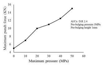
Fig. 16. Maximum punch force against different chamber pressure of a bilayer conical cup.
