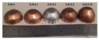
Fig. 8. Experimental samples without rupture.
