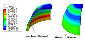
**Fig. 2.** Plastic strain of simulated bilayer conical cup drawing of ratio=2.2.
