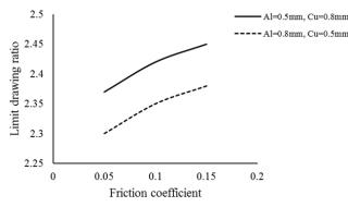
Fig. 12. Effect of coefficient of friction between punch and sheet on LDR of a bilayer conical cup.
