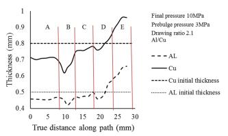
**Fig. 11.** Thickness distributions of the both layers for a bilayer conical cup.
