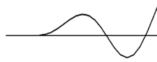
Fig. 11. Third vertical mode shape of third beam problem resulting from numerical simulation
