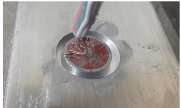
Fig. 14. Specimen after measuring the residual stresses by the ring-core method.
