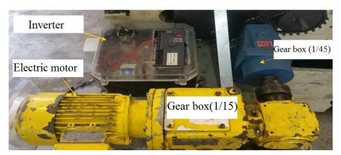
Fig. 1. Moving system of longitudinal feed for the grinding machine.
