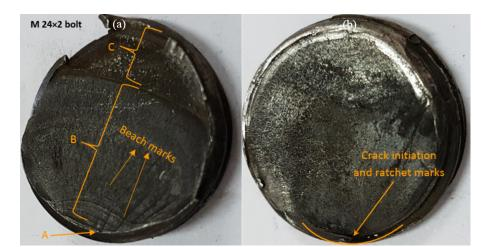
Fig. 7. Macro morphology of fracture surface of the radial forging machine bolts threads (zone 2).
