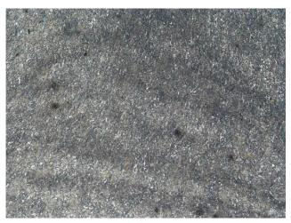
Fig. 4. Microstructure of the cross-sectional area of the base plate bolt after etching with  $100 \times$  magnification.
