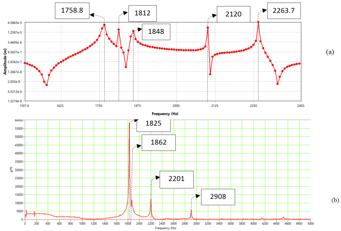
Fig. 10. Frequency response function diagram of healthy GFRP pipe obtained by a) Finite element simulation method, b) Experimental modal analysis method for the first and second natural frequencies.
