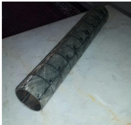
Fig. 1. A view of the GFRP pipe and its cross-sectional area.
