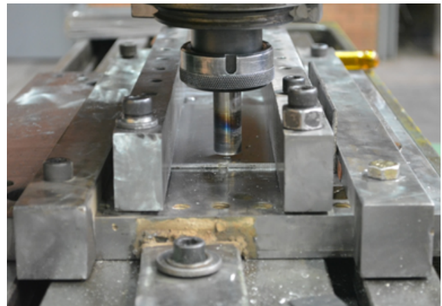
Fig. 1. Plate positioning and the FSW process.
