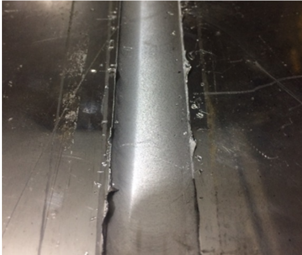
Fig. 2. Appearance of a sample friction stir welded Al-Al joint.
