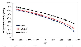
Fig. 3. The effects of the temperature on the dimensionless frequency of the SSSS piezoelectric rectangular micro-plate; a/b = 1, a/h = 20,  $V_0 = 200$ V.
