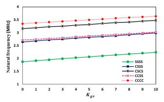
Fig. 5. The effects of the orthotropic Pasternak foundation and various boundary conditions on the dimensionless frequency of the piezoelectric rectangular micro-plate.
