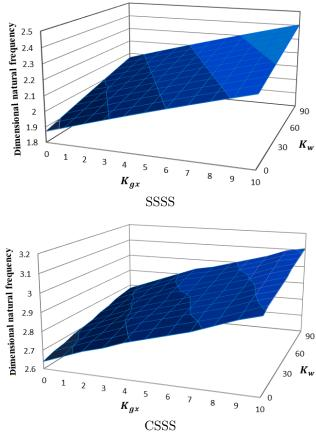
**Fig. 6.** The effects Winkler constant  $(K_w)$  and  $K_{gx}$  on the dimensionless frequency of the piezoelectric rectangular micro-plate corresponding to different boundary conditions.
