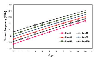
Fig. 4. The effects of the orthotropic Pasternak foundation on the dimensionless frequency of the SSSS piezoelectric rectangular micro-plate.
