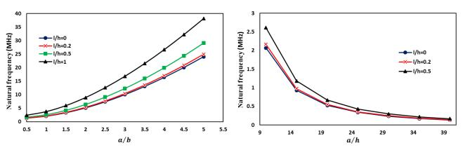
Fig. 2. Natural frequency of the rectangular micro-plate for SSSS boundary condition versus various, a) Aspect ratio (a/b), and b) Various length to thickness ratio (a/h).
