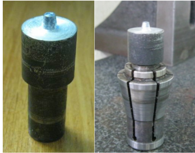
Fig. 1. The prepared H13 steel tool for welding.
