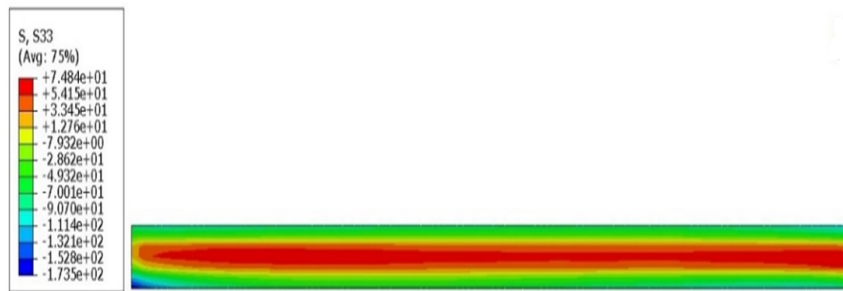
Fig. 5. Two-dimensional contour of residual stress on the cutting surface perpendicular to the grooves for CGP process obtained from ABAQUS software (1 st pass of CGP as a sample).
