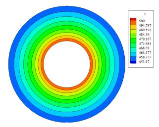
Fig. 5. Temperature distribution in the long cylindrical tube by the proposed code.
