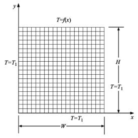
**Fig. 2.** The geometry shape of a thin rectangular plate under heat transfer and boundary conditions governing it.
