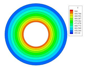
Fig. 6. Temperature distribution in the long cylindrical tube by ABAQUS.
