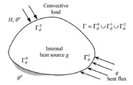
**Fig. 1.** Heat transfer problem modeling for threedimensional solid material [16].
