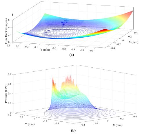
Fig. 4. The pressure distribution and film thickness in contact area for 200N load and 0.8m/s velocity.
