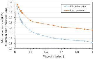
Fig. 7. Grease film thickness and maximum pressure to plastic viscosity,  $\phi$ .
