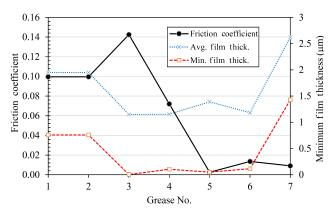
Fig. 5. Friction coefficient and film thickness for various type of lubricants, at 100N load and 1m/s entraining velocity.
