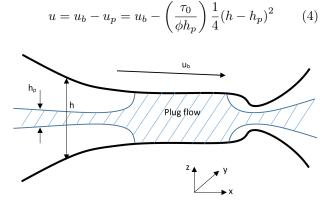
**Fig. 1.** Contact geometry in elastohydrodynamic lubrication and non-Newtonian grease lubricants.
