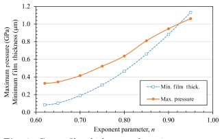
**Fig. 6.** Grease film thickness and maximum pressure to rheological exponent, *n*.
