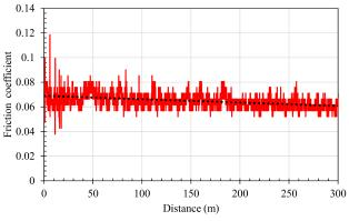
**Fig. 3.** Experimental results of friction coefficient in 20N load and 0.23m/s velocity condition.
