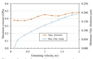
Fig. 9. Speed effect on film thickness and maximum pressure.
