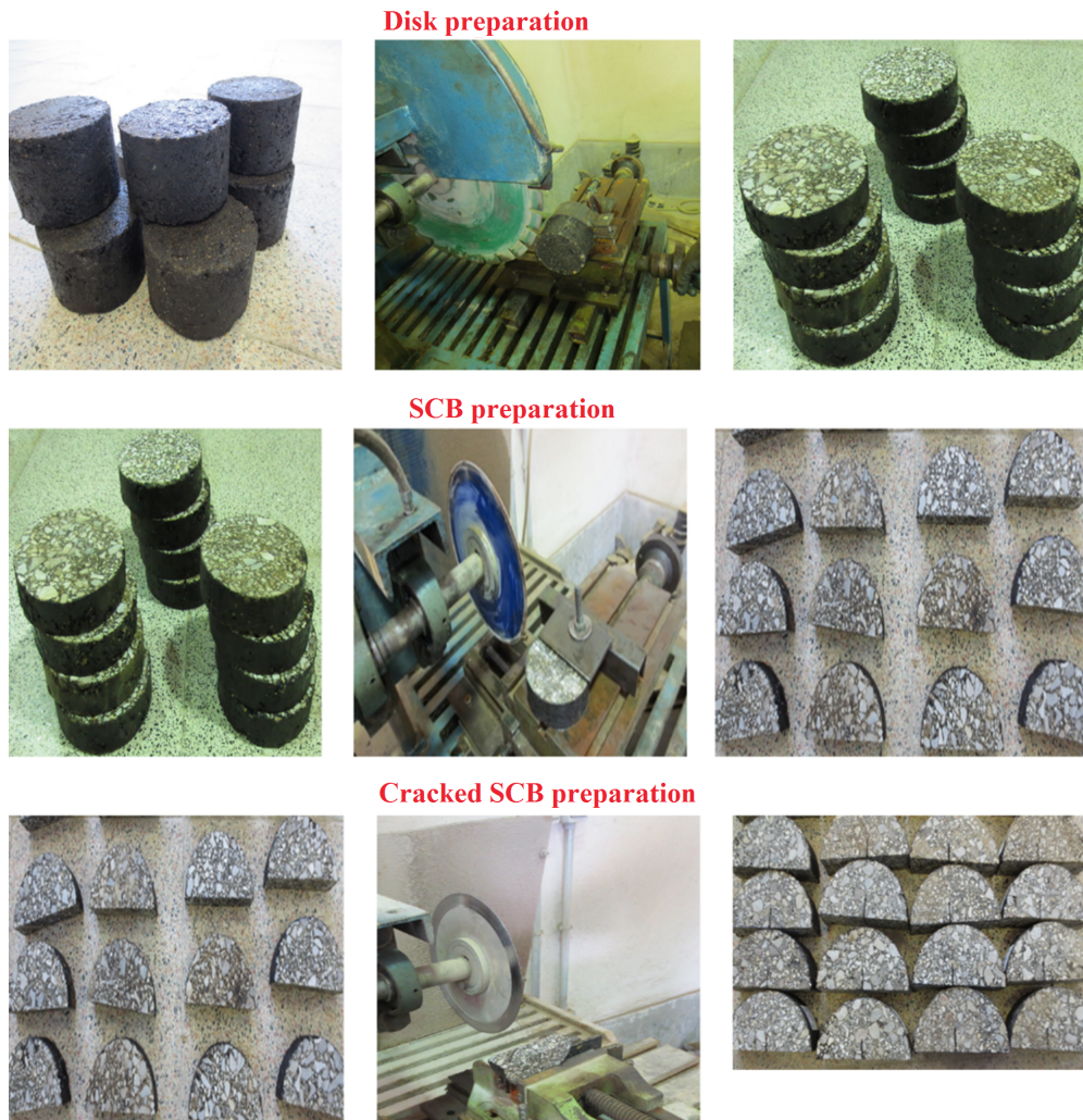
Fig. 3. Steps of producing SCB specimens.
