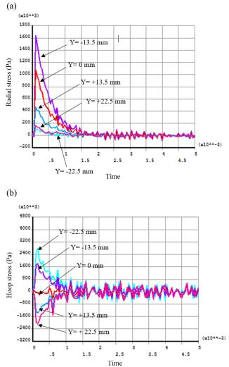
Fig. 8. The values of time historical of a) Radial, b) Hoop stresses for nodes located at (X = 100 mm, Z = 0) and  $Y = \pm 22.5$  mm, 13.5 mm, 0 mm.
