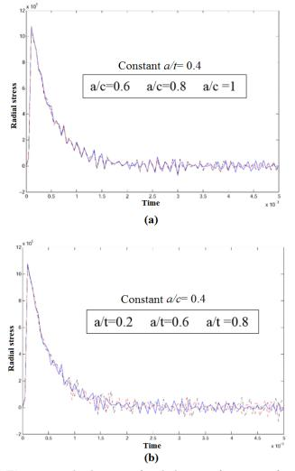
Fig. 10. The history of radial stress for points far away the defect location in cylindrical vessels with different crack profiles, a) Constant  $\eta = 0.4$ , and different  $\xi = 0.6, 0.8$  and 1; b) Constant  $\xi = 0.4$  and different  $\eta = 0.2, 0.6$ , and 0.8.
