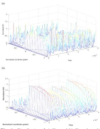
**Fig. 5.** Distribution of a)  $K_{II}$  and b)  $K_{III}$  through the crack line vs. time for a semi elliptical shape defect with  $\xi = \eta = 0.4$ .
