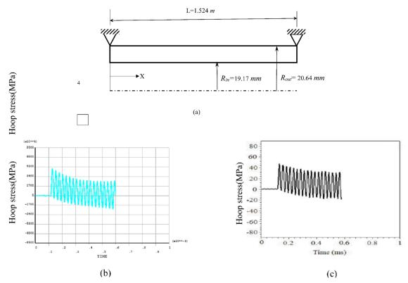
Fig. 3. The hoop stress versus time at X = 0.3038 m from the ignition side of a 2d tube under denotation, a) Schematic representation of detonation tube, b) Finite element prediction, c) Transient analytical approach results.
