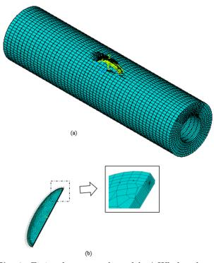
**Fig. 2.** Finite element mesh model; a) Whole volume, b) Crack region.
