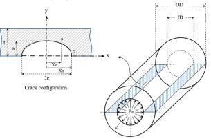
Fig. 1. The schematic diagram of a cylindrical pressure vessel with an embedded elliptical defect.
