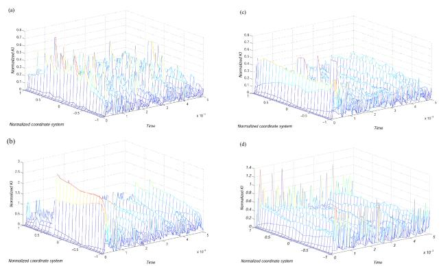
Fig. 4. Variation of  $K_I$  along the crack front versus time for constant  $\xi = 0.4$  and different crack depths i.e., a)  $\eta = 0.2$ , b) 0.4, c) 0.6, d) 0.8.
