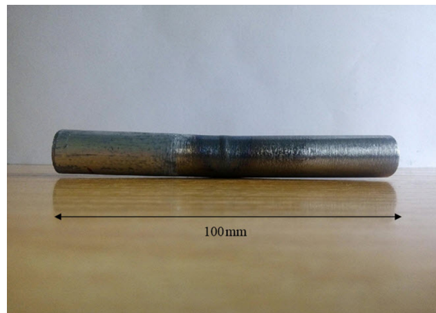
Fig. 1. A laser-bent tube with the laser beam in the experiments.
