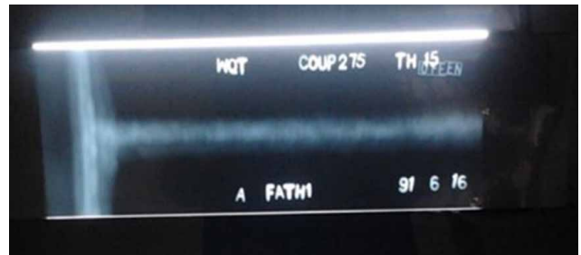
Fig. 2. Radiographic image of a super-duplex steel pipe welding sample.
