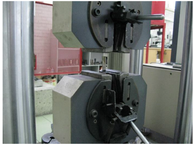
Fig. 3. Tensile-shear test of resistance spot welded AISI 304 sheets.
