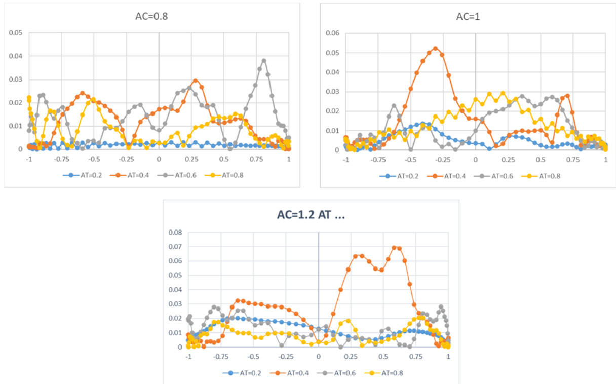
Fig. 18. Distribution of the stress intensity coefficient in mode II along the front of the semi-elliptical crack ( a/c = 0.8, 1, 1.2 , Different a/t values).
