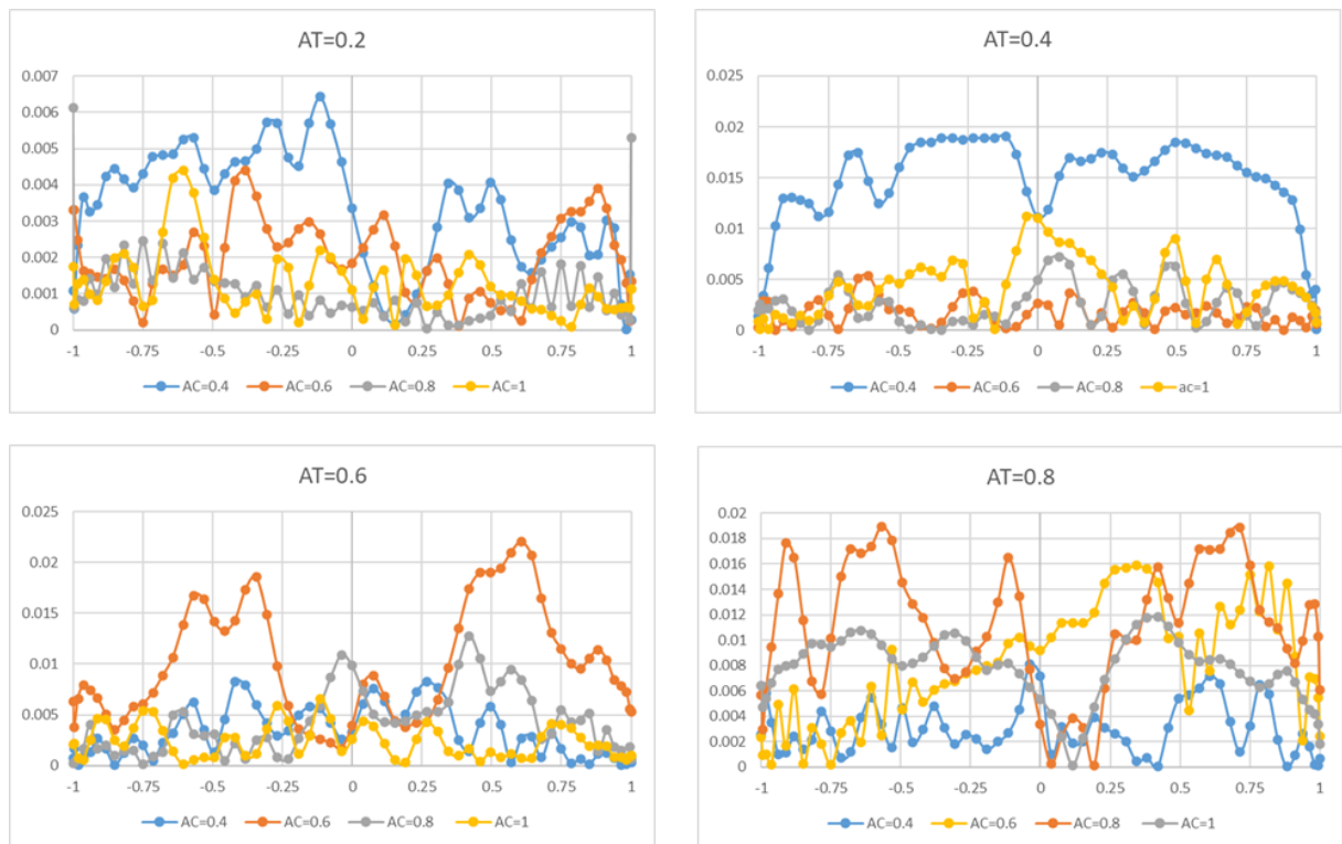
Fig. 19. Distribution of the stress intensity coefficient in state III in the semi-elliptical crack front extension (constant a/t = 0.2, 0.4, 0.6, 0.8 , and different a/c ).
