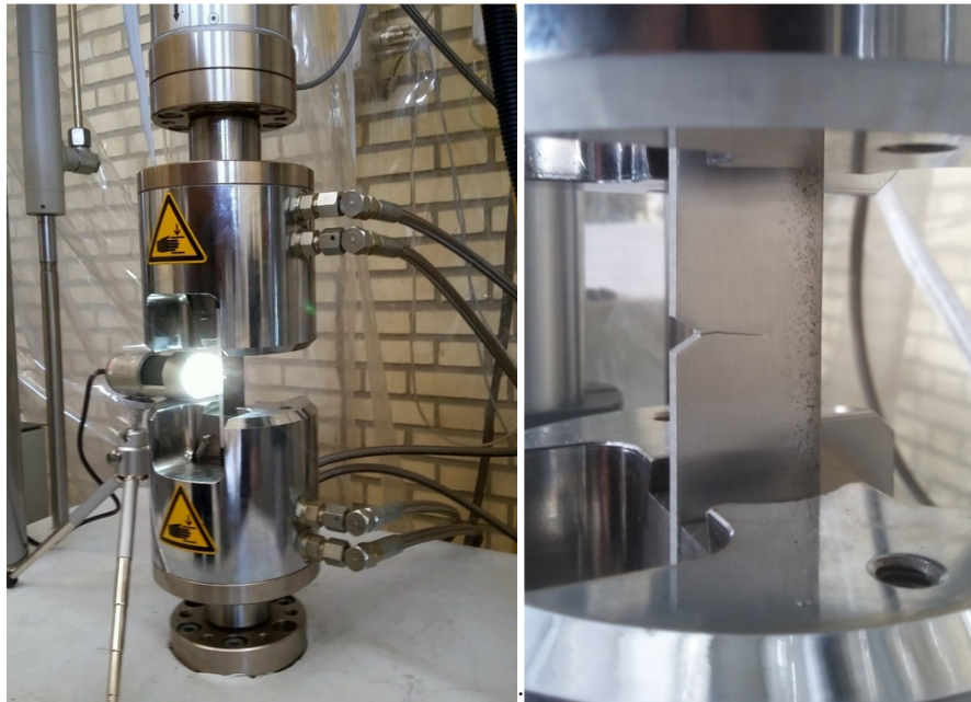
Fig. 4. The assembled specimen on the testing machine and a cracked sample.
