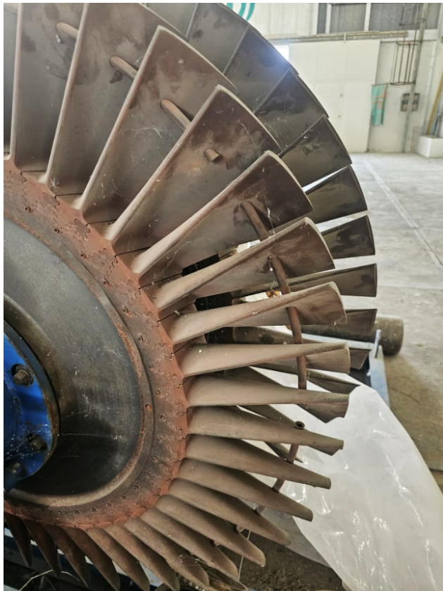
Fig. 2. View of an undamaged power turbine.
